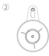
Turn counter clockwise to open the battery cover
